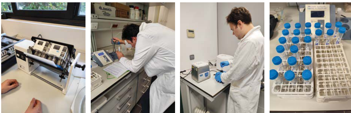
Photos 15 to 18. Laboratory analysis of soil pH and electrical conductivity
