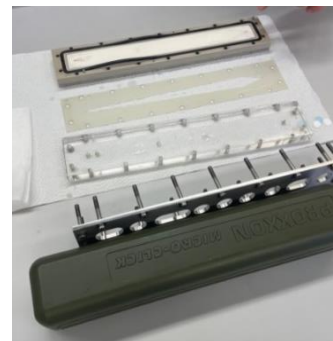
Figure 4. Preparation of the membrane of the separation channel/filter/loop
