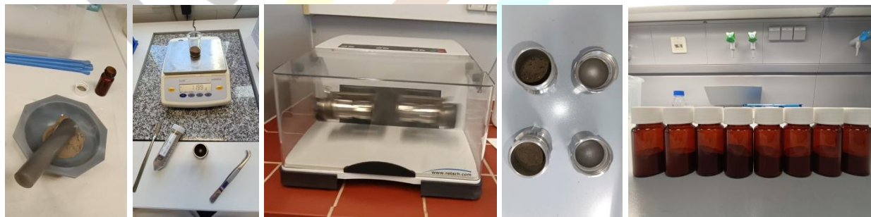
Figure 9. Sample preparation for X-ray diffraction analysis and electron paramagnetic resonance spectroscopic analysis
