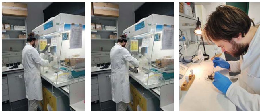
Photos 35 to 37. Treatment of soil samples with hydrofluoric acid and subsequent separation of organic matter
