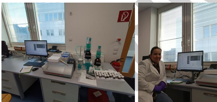
Figure 8. DLS analysis using Litesizer 500
