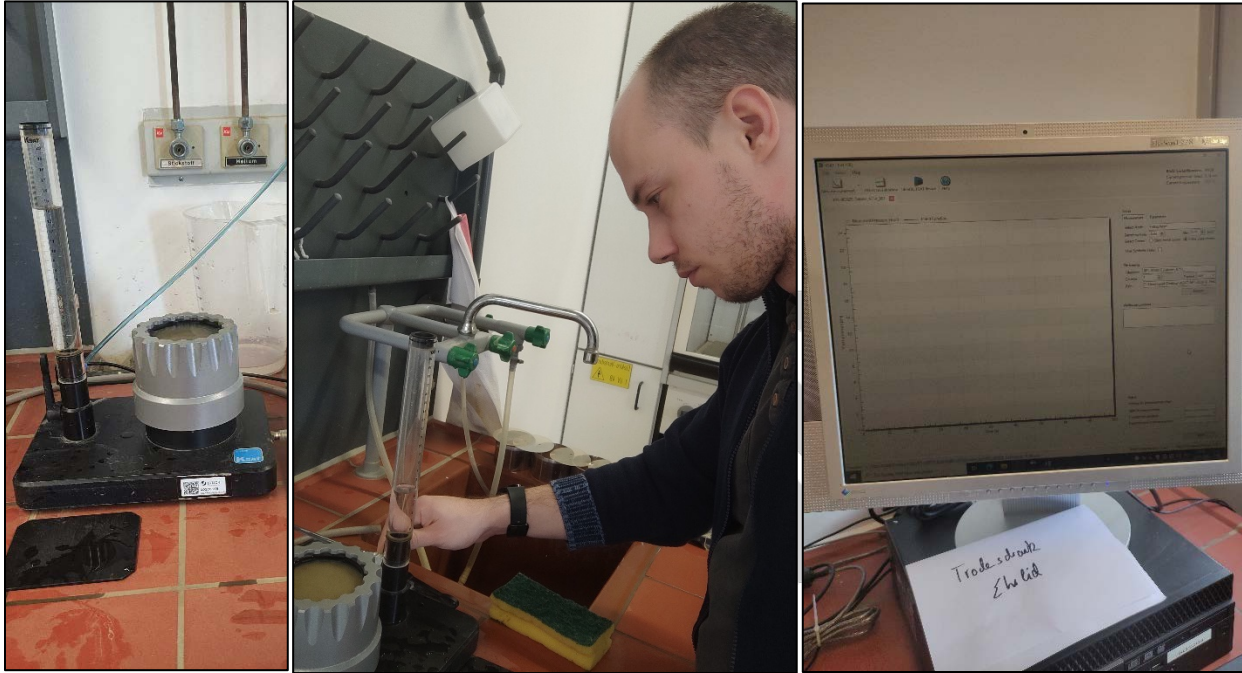
187 188 Figure 10. Measuring saturated hydraulic conductivity of all soil (mixture) samples using the 189 KSAT Device (Meter Group, Munich) 190
