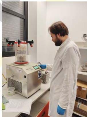
Photos 38 and 39. Initiating the lyophilization process for soil samples
