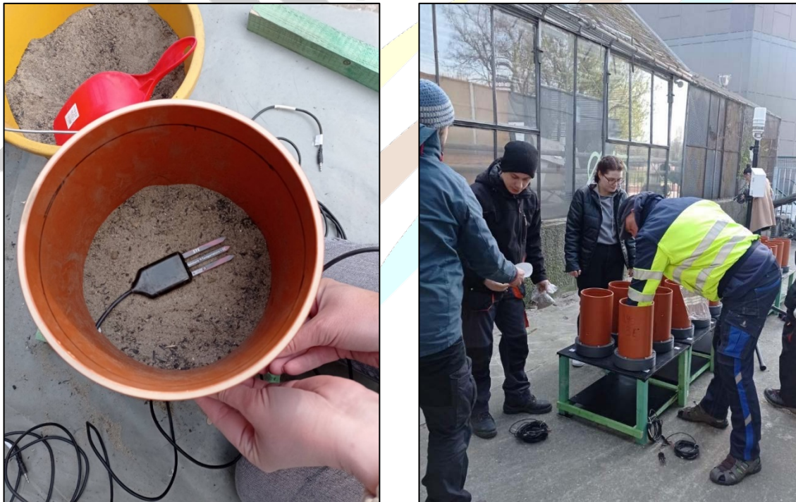
Figure 3. Placing sensors and connecting to loggers
