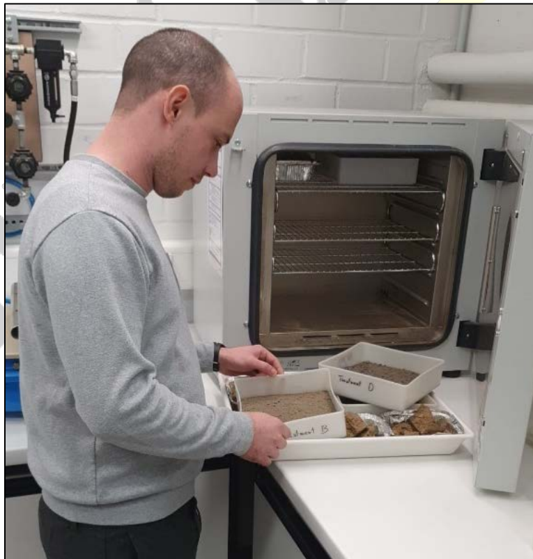
Figure 7. Drying of soil samples in laboratory oven prior to hydraulic characterization
