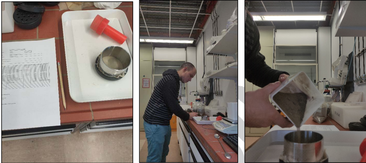
174 Figure 8. Determination and weighting of soil mixture samples based on corresponding bulk 175 density
