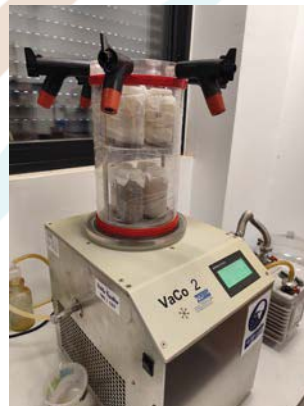
Photos 38 and 39. Initiating the lyophilization process for soil samples
