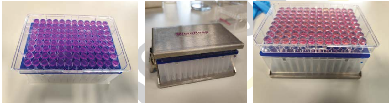
Photos 32 to 34. Setup of the detection plate and vacuum sealing for incubation, and opening after 6 hours for spectrophotometric reading
