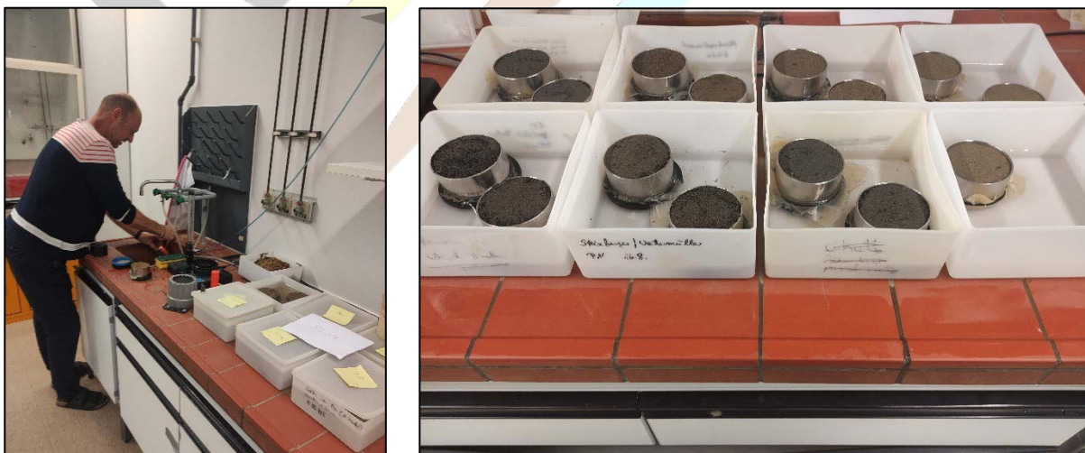
184 Figure 9. Packing soil into cylinders and appearance of filled cylinders during the saturation 185 process 186
