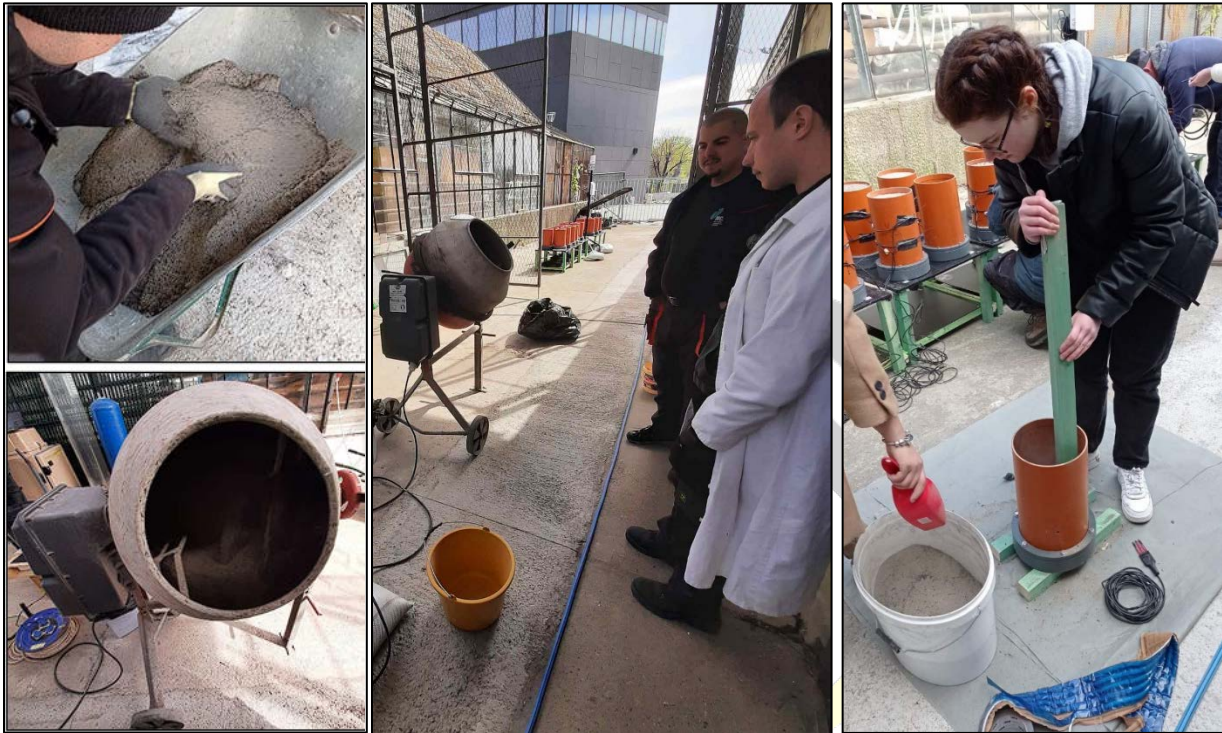
Figure 2. Mixing of materials, filling (and compacting) of lysimeters
